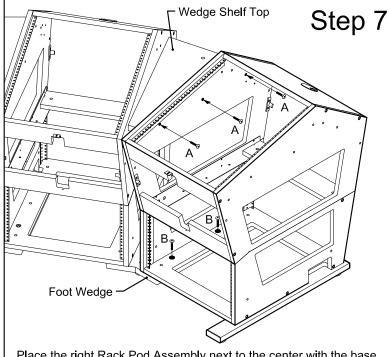
Place the right Rack Pod Assembly next to the center with the base resting on the Foot Wedge. Attach the Wedge Shelf Tops to the center Rack Pod as shown with 55mm x 1/4"-20 connector bolts(A). Attach the right Rack Pod Base to the Foot Wedge with 40mm x 5/16"-18 connector bolts. Repeat this assembly for the left side.
